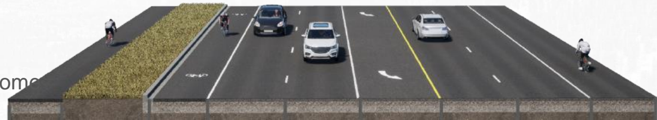
Example of a five-lane cross section, matching SR-248 west of Richardson Flat Road
