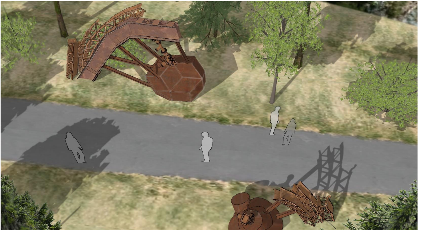
Figure 2: Aerial view. Steel hollow-forms serve as pour-forms for reinforced concrete to support the structure.
