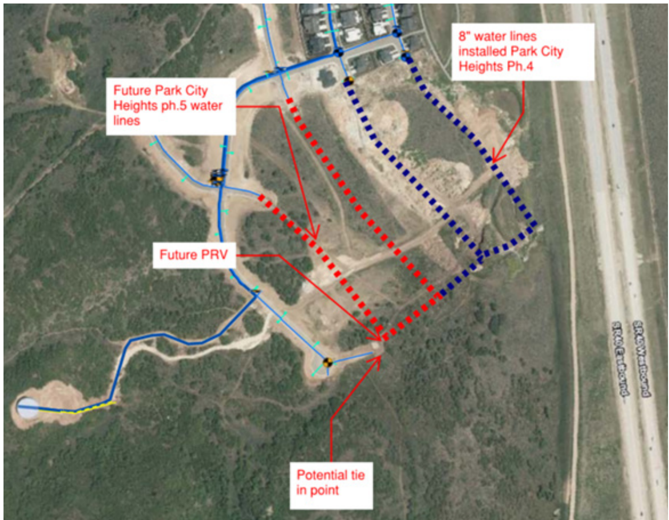
Illust. 171 - Conceptual Water Connection layout
