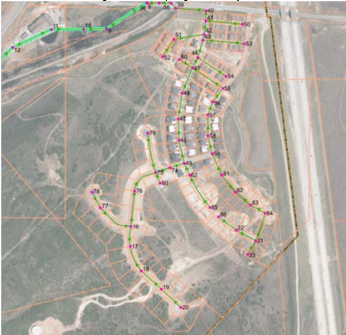
Figure 2 – Park City Heights Sewer Layout
