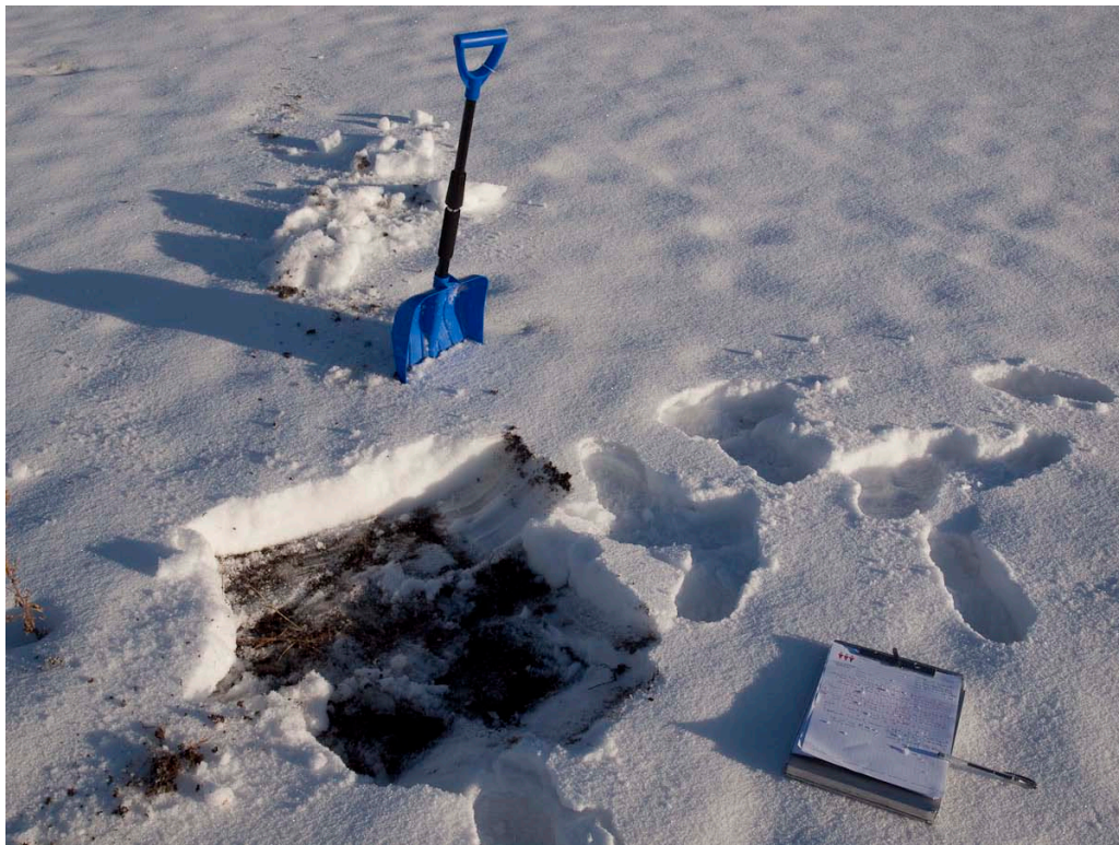
Photograph 1. Use of a collapsible shovel to sample vegetation under the snow pack.
