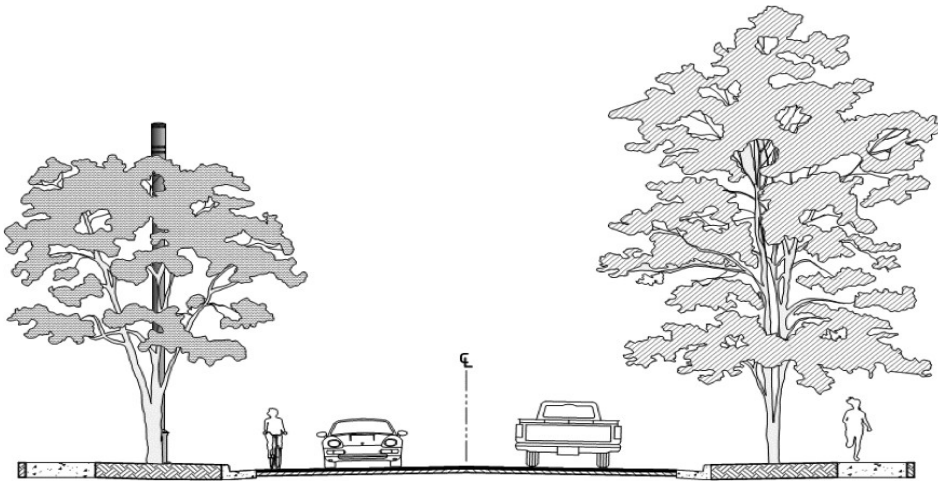
Figure 6-3: Freestanding Pole SWF in City ROW
