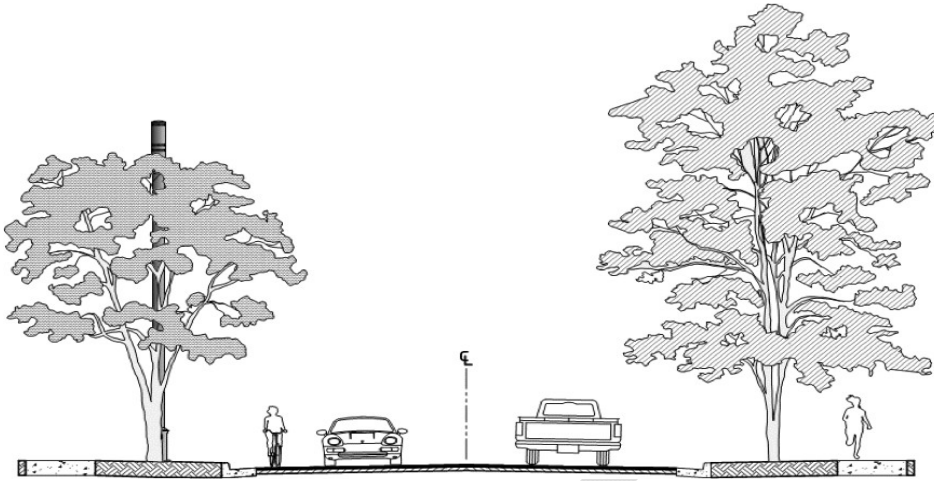
Figure 6-3: Freestanding Pole SWF in City ROW
