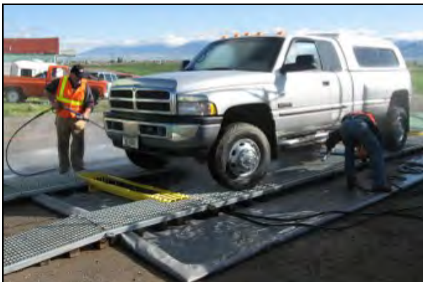
Portable vehicle cleaning stations prevent transportation of noxious weed seed to new location.
