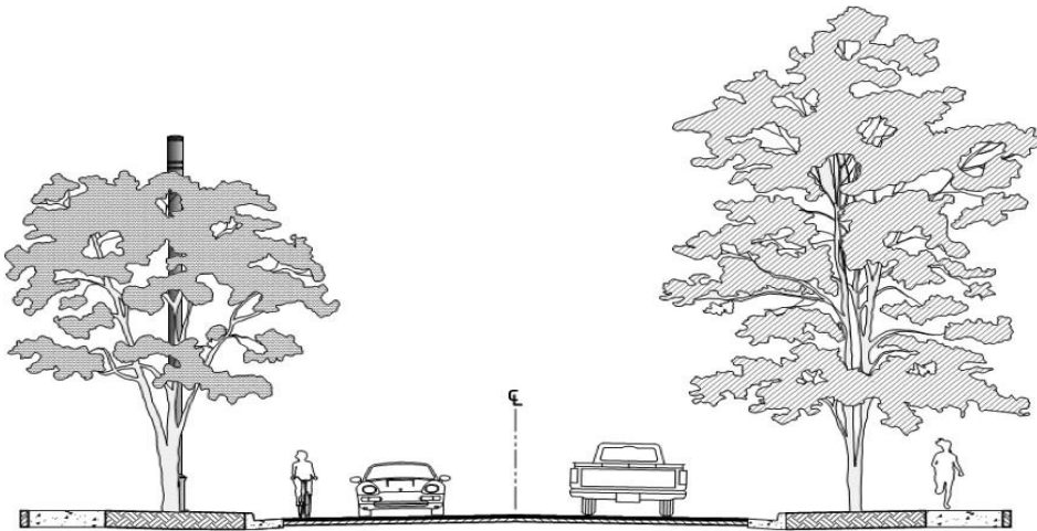
Figure 6-3: Freestanding Pole SWF in City ROW
