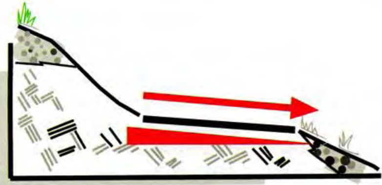
Outslope helps water sheet across and off the trail
