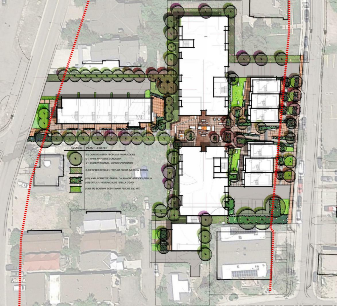
Figure 8: Excerpt from Sheet A901.7. Red dashed line identifies the as-measured 20 foot (20') Front Yard Setback line for the entire streetscape shown.
