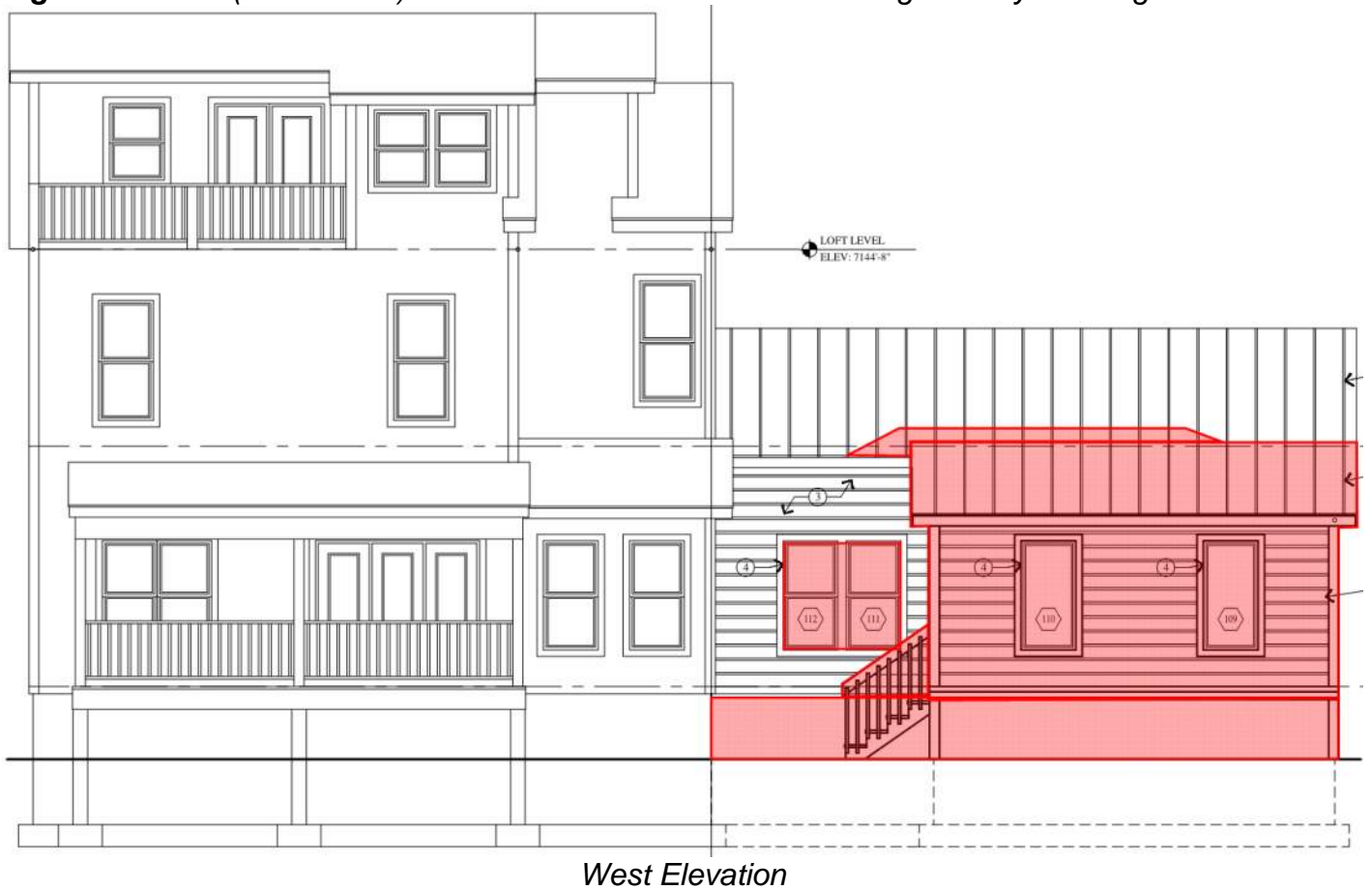
Figure 2: Areas (shaded red) that are to be removed from the single-family dwelling
