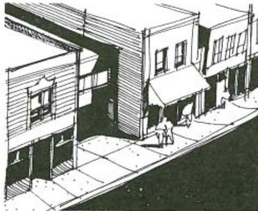
Alignment at sidewalk edge not respected.
