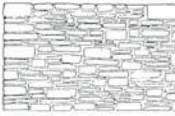
Squared Rubble A rubble wall built of squared stones of varying sizes and coursed at every third or fourth stone.
