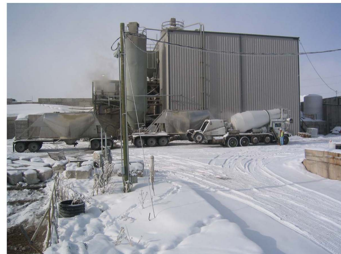
Comparison of Cement Delivery Truck Versus Concrete Mixer Truck
