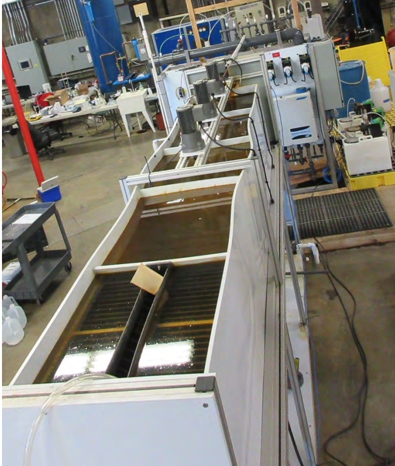
Figure 3-4: Flocculation and Sedimentation Skid From Above
