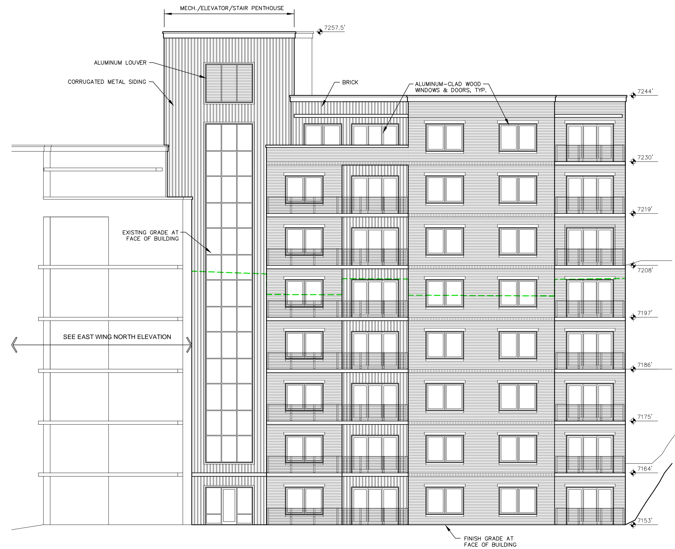
WEST WING - NORTH ELEVATION
