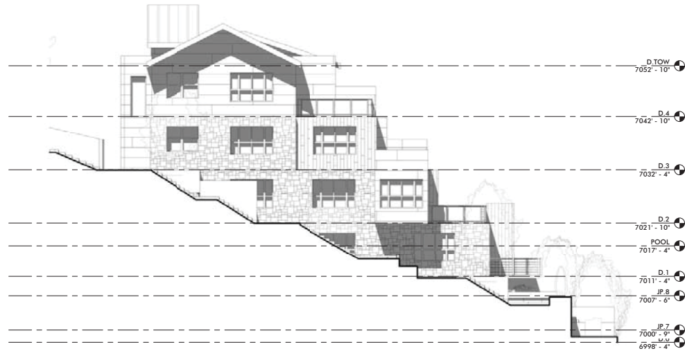
2 BUILDING D SOUTH ELEVATION SCALE: 1/8" = 1'-0"
