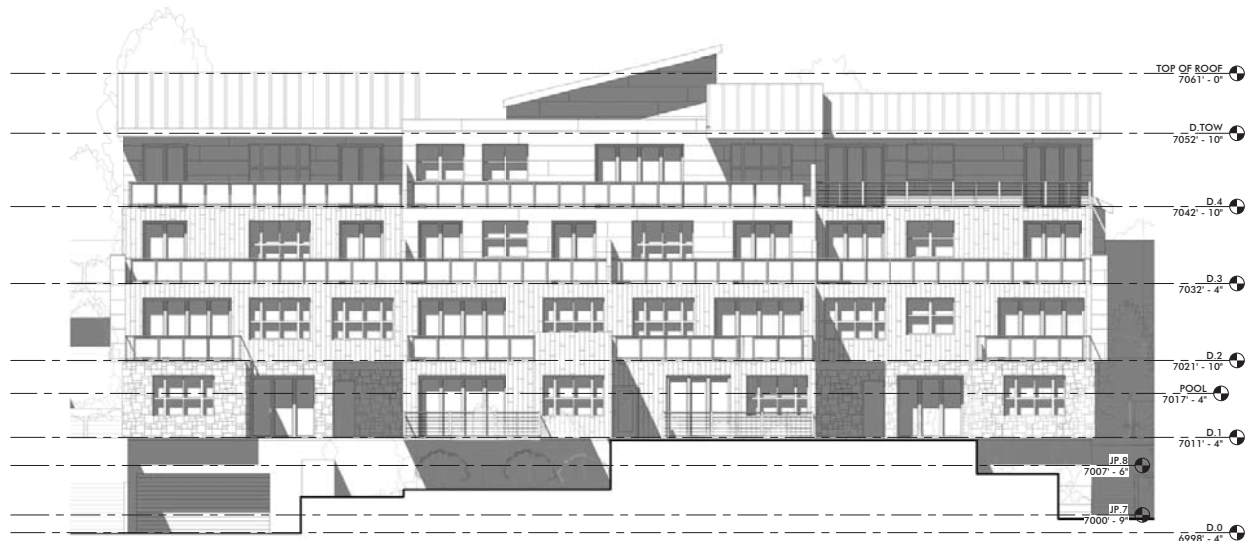
① BUILDING D EAST ELEVATION SCALE: 1/8" = 1'-0"
