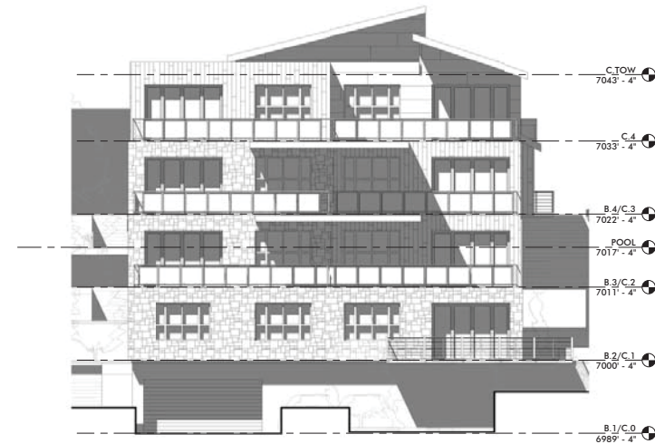
3 BUILDING C EAST ELEVATION SCALE: 1/8" = 1'-0"
