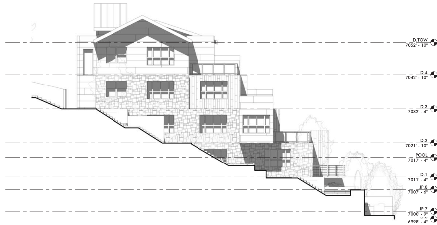
2 BUILDING D SOUTH ELEVATION SCALE: 1/8" = 1'-0"
