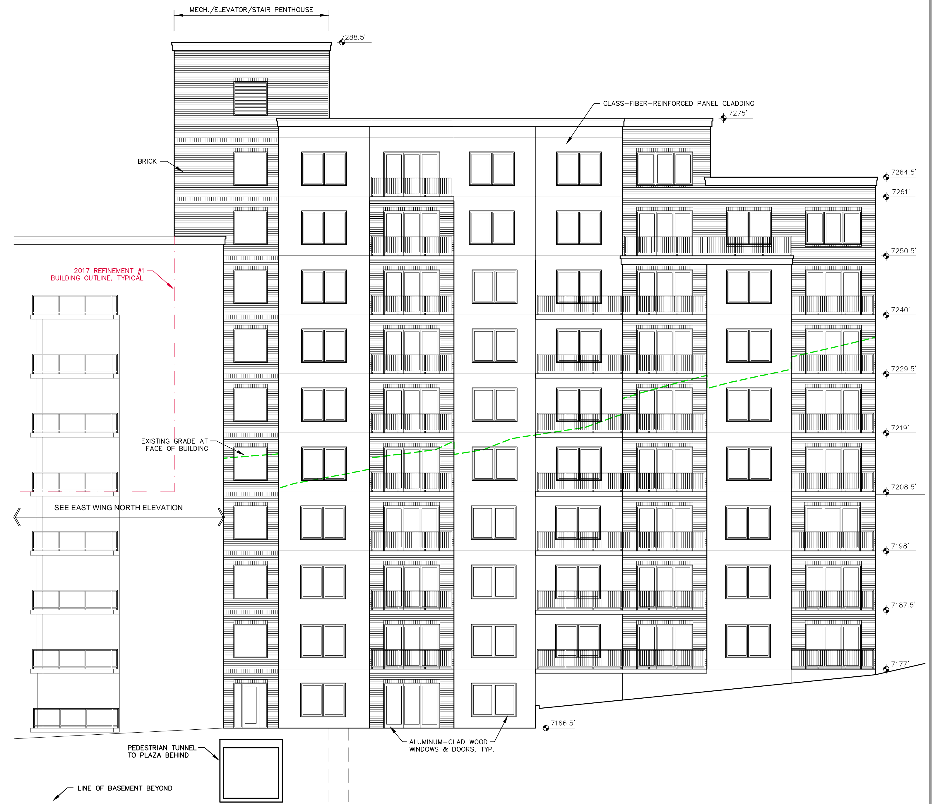
WEST WING - NORTH ELEVATION
