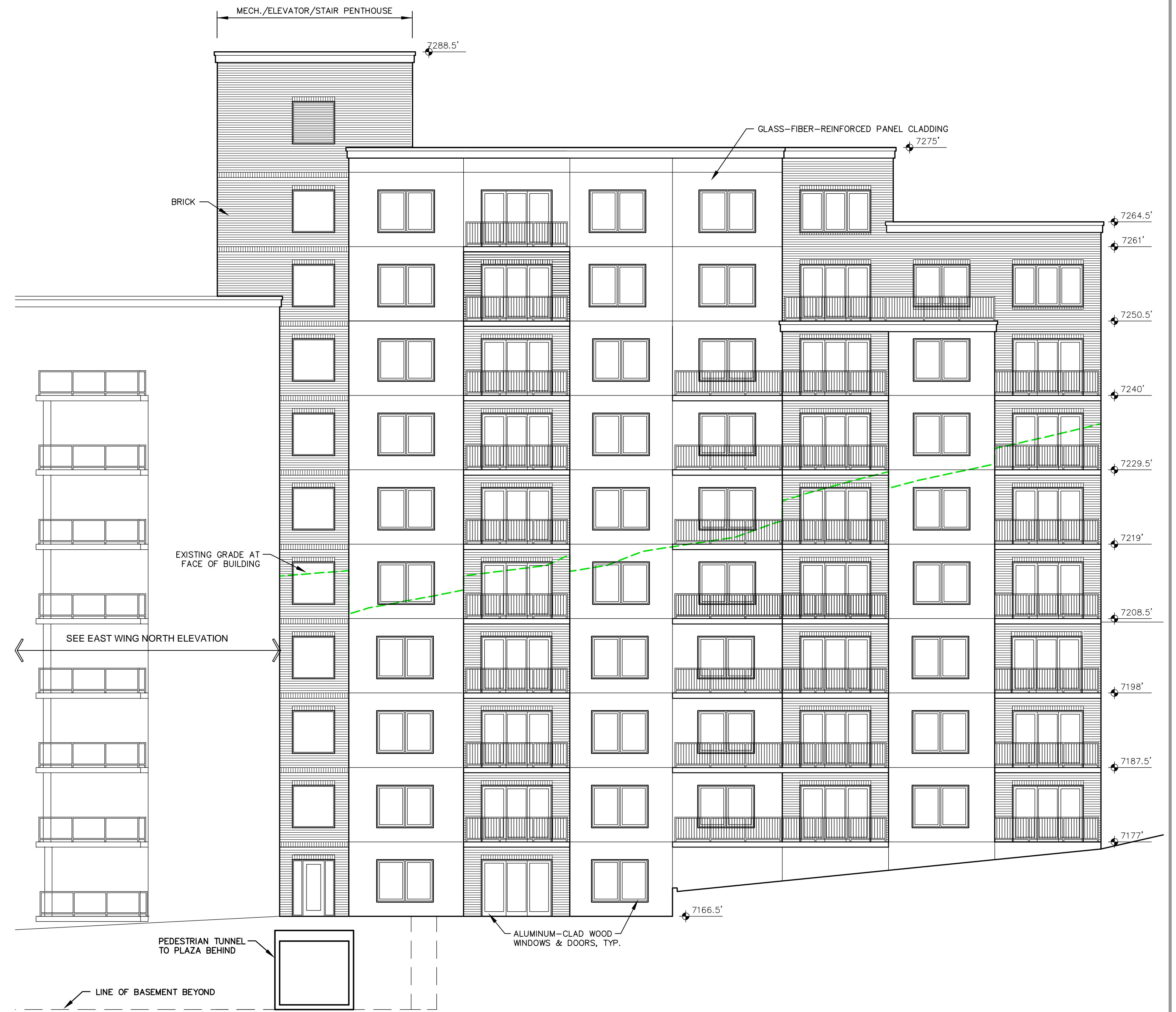
WEST WING - NORTH ELEVATION
