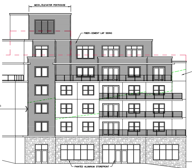
NORTHEAST ELEVATION - NORTH WING
