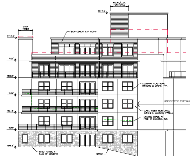
NORTHEAST ELEVATION - SOUTH WING
