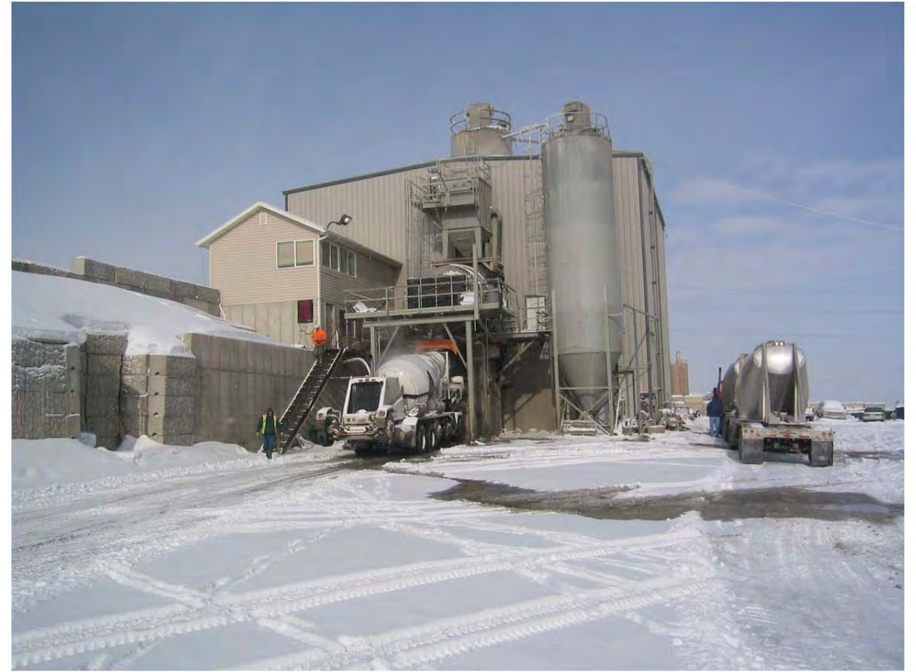
Loading Concrete Mixer Truck
