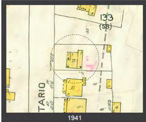
Sanborn Fire Insurance map shows the original L-shaped cottage with a one-story addition across the back. A partial-width front porch is adjacent to stem wing.
