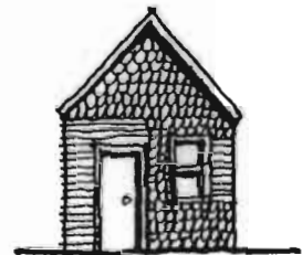
Too much ornamental siding.
