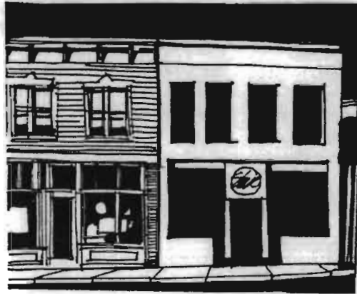
Traditional storefront components are retained in this new scheme.
