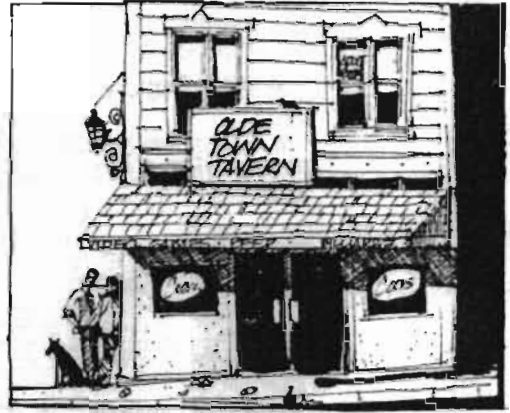
Inappropriate: Portions of the original facade concealed.
