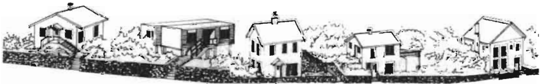
Shape of adjacent buildings not respected.
