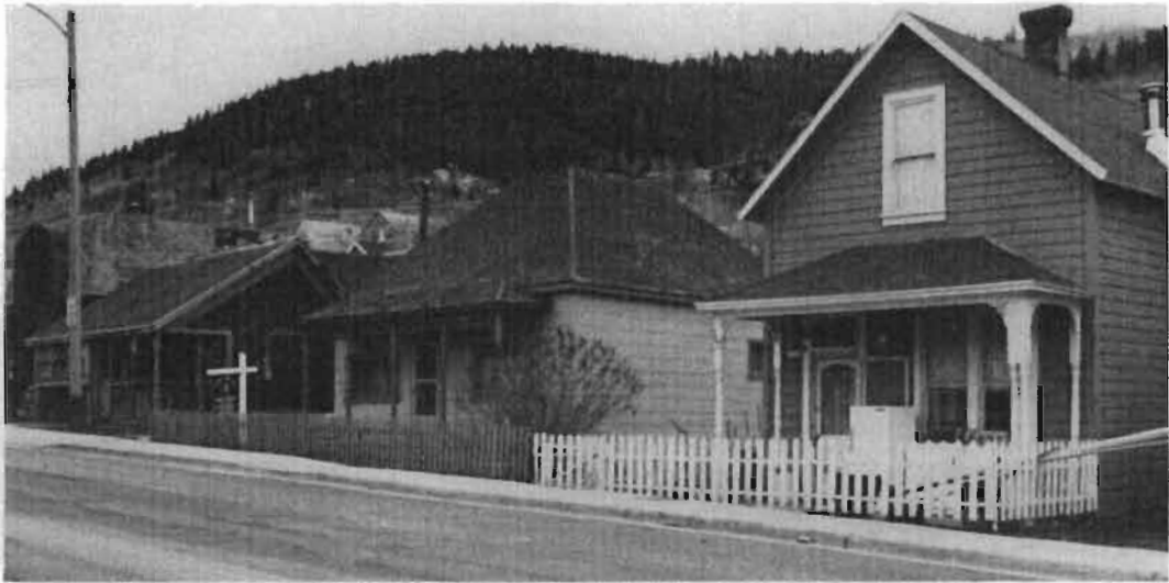
Even though the sizes and shapes of these facades vary, the pattern created by the porches unifies this row. The pattern is reinforced by equal porch widths, porch roof heights and uniform setbacks. Picket fences create another pattern.
