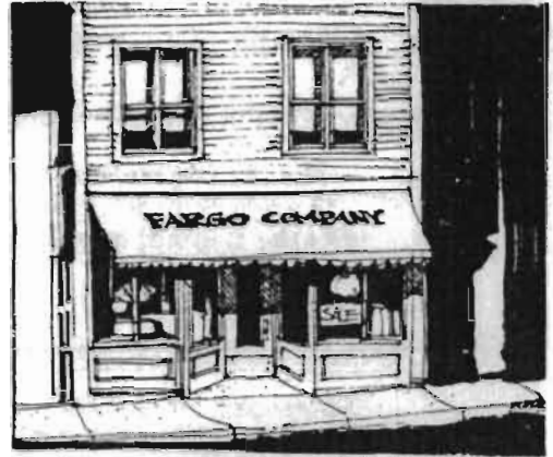
This awning is positioned properly because it fits the store width and does not cover the interim cornice.
