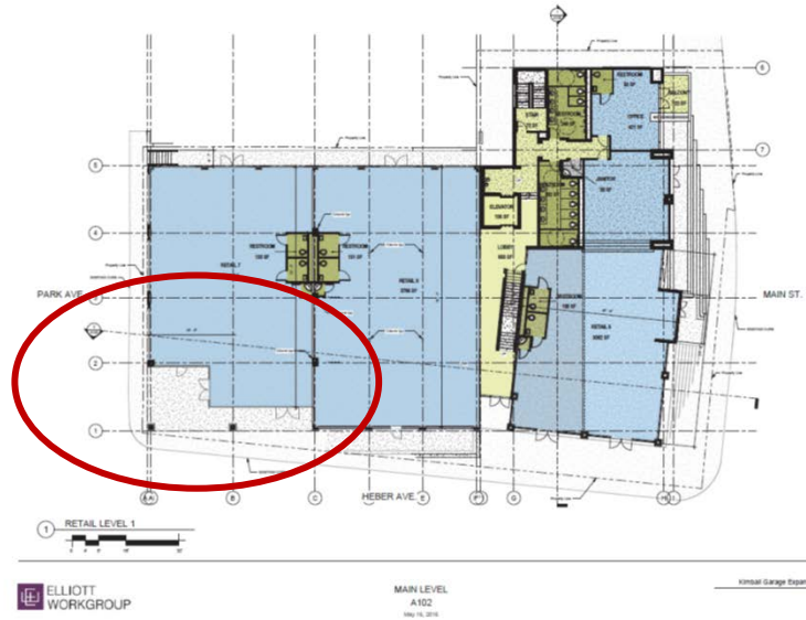
Figure 12. The area beneath the overhang on the west side of the building was enclosed early on as is evident in Figures 1 and 2. The divided-light glass addition beneath the overhang was constructed c.1976. The applicant is proposing to maintain the dimensions and transparency of the existing addition, though the window units will need to be replaced.
