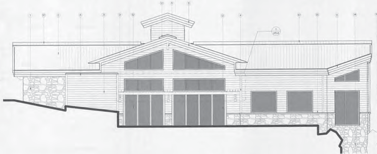
1 NORTH WEST ELEVATION A2.1 1/4" = 1'-0"
