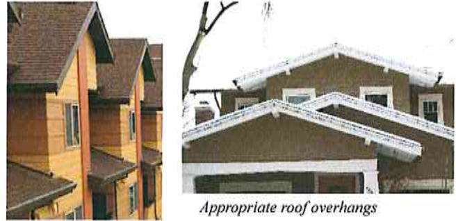
Overhangs protect walls
