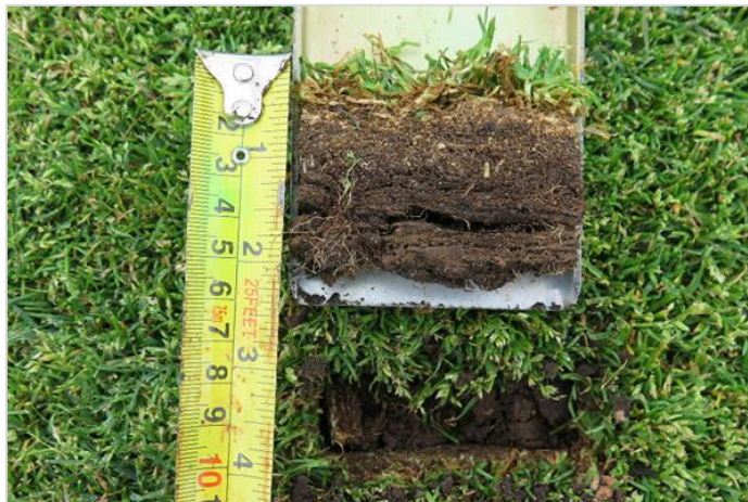
Soil profile sample showing the dense layer of thatch on top of the native material on fairways.
