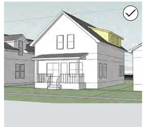
Figure 23: Location & Design of a Residential Addition
