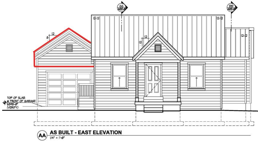
Diagram 5: The red outline shows the portion of the garage that will be removed.
