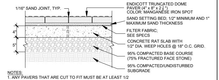
PEDESTRIAN TRUNCATED DOME BRICK PAVING - SECTION
