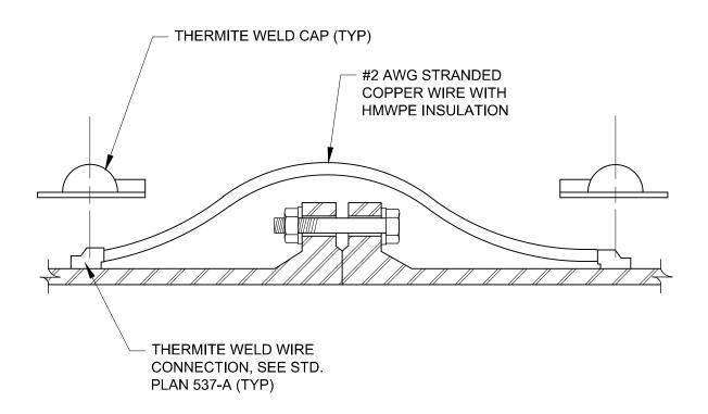
INSTALL TWO BOND WIRES AT EACH PIPE JOINT.
