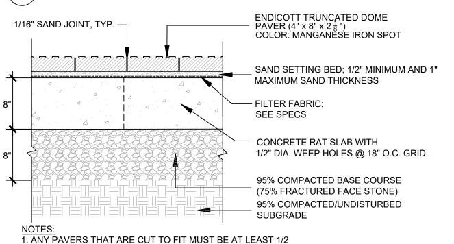
ANY PAVERS THAT ARE CUT TO FIT MUST BE AT LEAST 1/2 THE ORIGINAL 4"x8" PAVER
