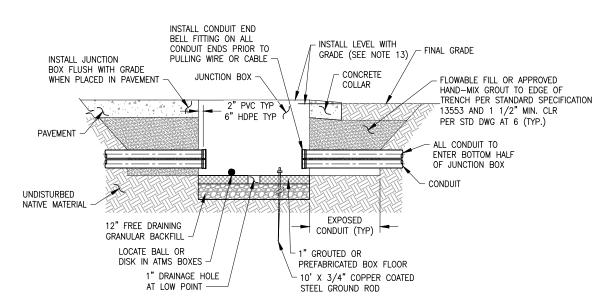
JUNCTION BOX CONDUIT PRENETRATION DETAIL
