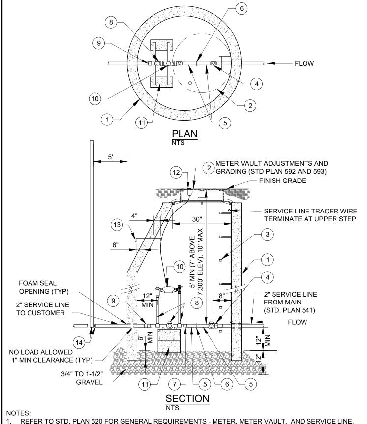
REFER TO STD. PLAN 520 FOR GENERAL REQUIREMENTS - METER, METER VAULT, AND SERVICE LINE.
