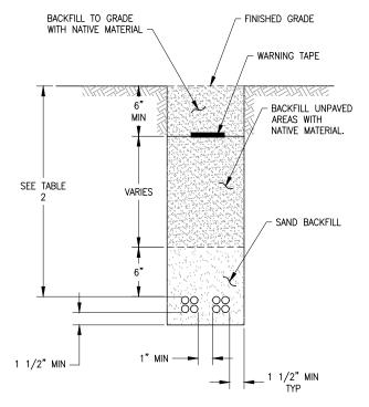
WARNING TAPE BACKFILL TO GRADE WITH NATIVE MATERIAL BACKFILL UNPAVED MIN AREAS WITH NATIVE MATERIAL. SEE TABLE VARIES SAND BACKFILL SEE TABLE VARIES - 1 1/2" MIN 88 88 88 1 1/2" MIN — 1 1/2" — 1 1/2" MIN -
