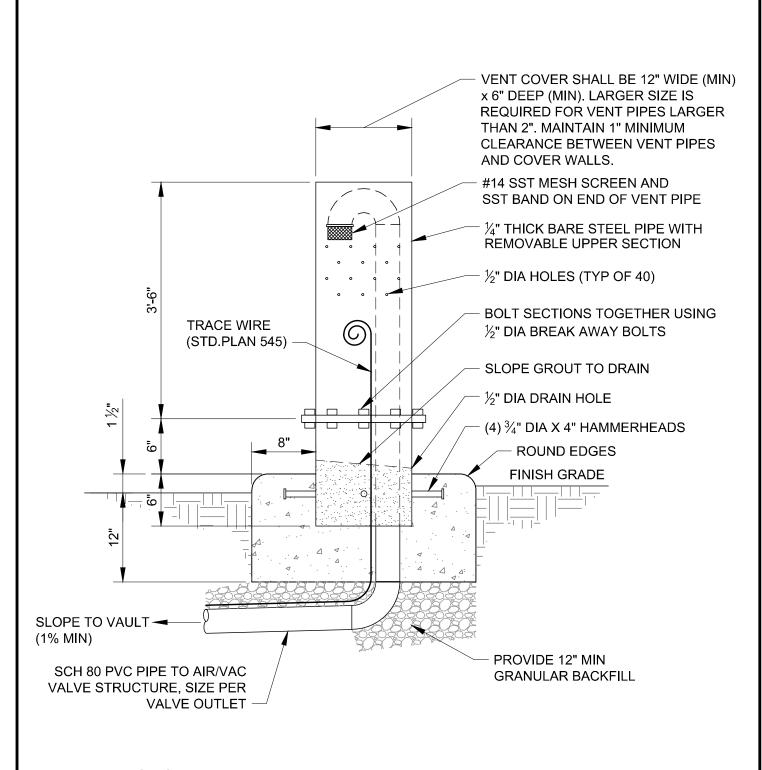
1. LOCATE VENT AS SHOWN ON APPROVED PLANS, 1'-6" MINIMUM BEHIND TOP BACK OF CURB / GUTTER OR SIDEWALK.
