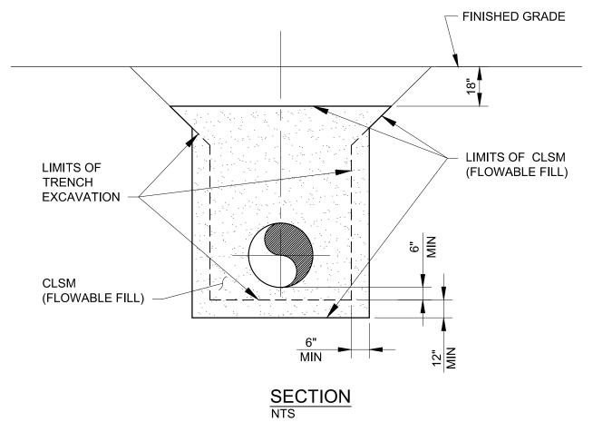
1. CLSM - CONTROLLED LOW STRENGTH MATERIAL, DESIGN MIX 100-150 PSI
