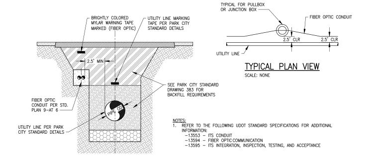
CONDUIT TRENCHED IN ASPHALT PAVEMENT RESTORED WITH T PATCH FIBER OPTIC CONDUIT IN COORDINATION WITH OTHER UTILITY INSTALLATION
