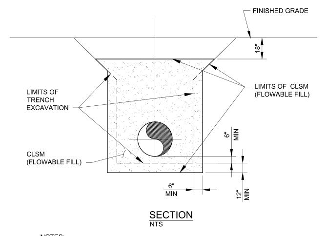
1. CLSM - CONTROLLED LOW STRENGTH MATERIAL, DESIGN MIX 100-150 PSI
