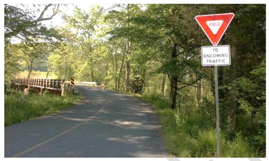
Figure 8: Example of Yield Sign and Supplementary Plaque – Hana Highway in Maui, HI
